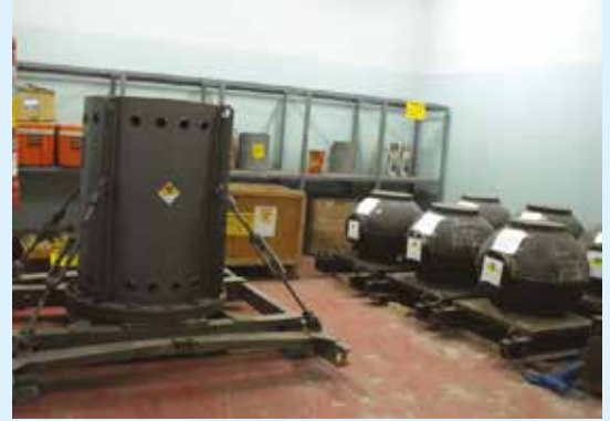
Storage of Disused Sealed Radioactive Source at CWPSF
